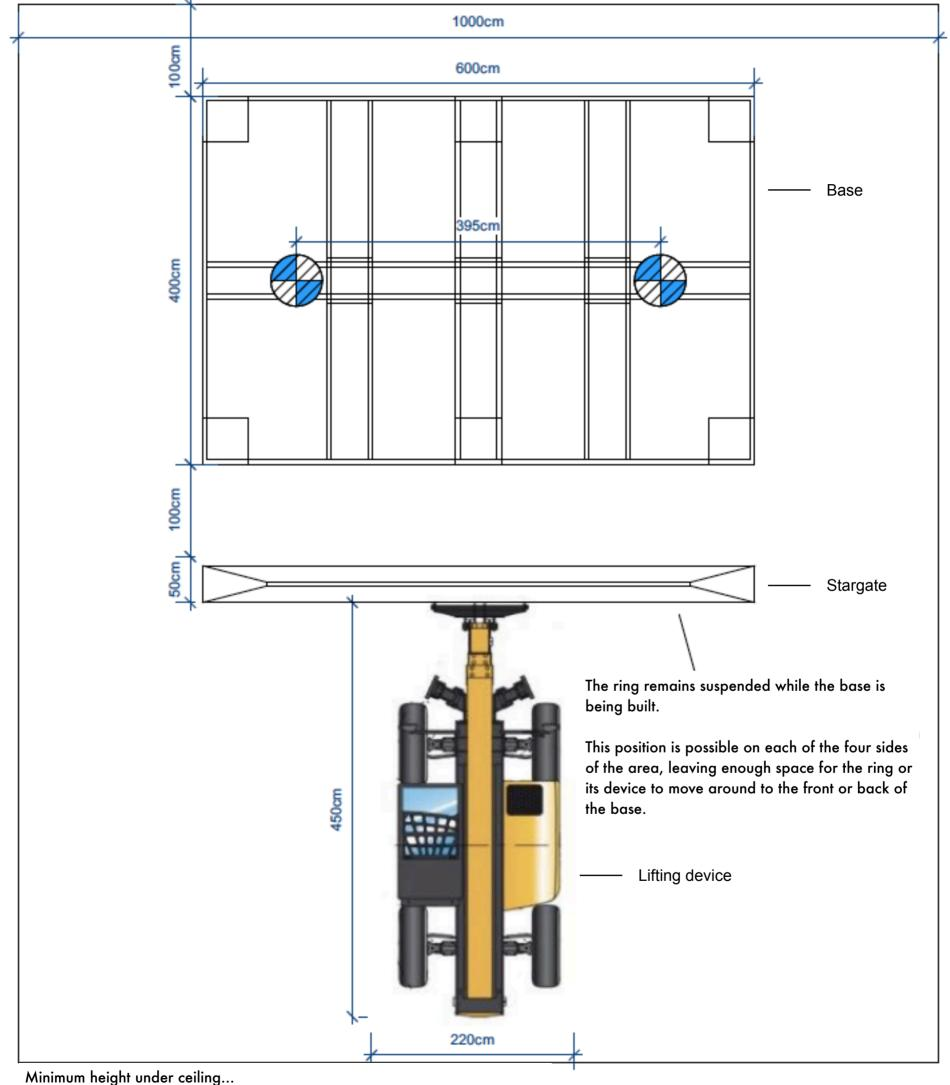
Lifting with motorized device: 8m Lifting with hoists: 7.5m Total weight : 1t Capacity of each attachment point 1 ton (with a safety coefficient of 2x)
