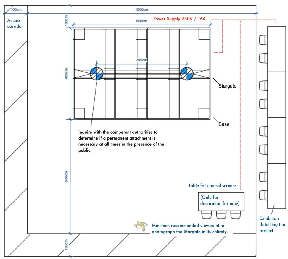
Minimum height under ceiling... Lifting with motorized device: 8m Lifting with hoists: 7.5m
